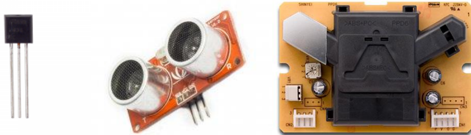
Figure 2. Examples of sensing devices (left to right): Parallax temperature 56 , Arduino distance 57 , and Shinyei particle sensor 58 (air pollution).
