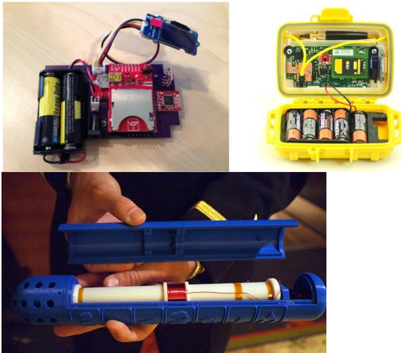
Figure 3. Examples of sensor hardware: Noise monitor 59 (left), SweetSense™ 60 (right), and HealthyShrimp 40,41,61 (bottom).
